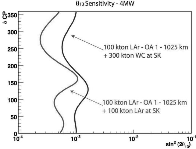
**Fig. 7**  $\theta_{13}$  sensitivity at  $3\sigma$  C.L. for a two detector configuration. A 100 kton LAr detector is located at 1025 km, 1 degree off-axis and a second detector i.e 300 kton WC (blue line) or 100 kton LAr (red line) is located at SK.
