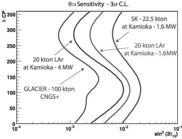
**Fig. 5**  $\theta_{13}$  sensitivity at  $3\sigma$  C.L. for 20 kton LAr detector at 295 km, 2.5 degrees off-axis for 5 years of neutrino beam at 1.6 MW (green line) and 4 MW (blue line). For comparison the sensitivity of T2K (22.5 kton WC at Kamioka - 1.6 MW) and GLACIER-100 kton on upgraded CNGS [13] are given.
