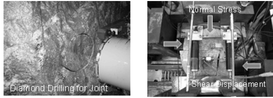
Fig. 6 Situation of core drilling and direct shear test for joint.
