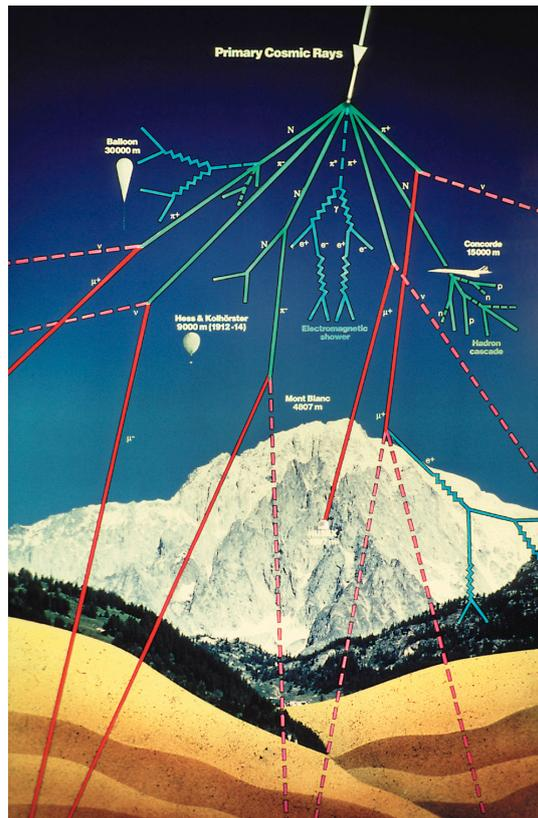
Figure 5: A schematic representation of a primary cosmic ray collision and shower in the atmosphere. [65]
