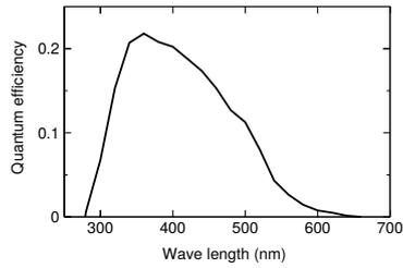
Figure 12: Example distribution of the quantum efficiency of a PMT photocathode (used in Super-Kamiokande). [4]
