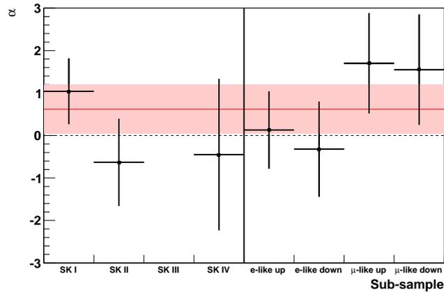
Figure 72: The best-fit  $\alpha$  parameter obtained by performing the analysis on sub-samples of the data, showing SK periods on the left, and data sub-sample types on the right. The red band shows the combined result. The SK-III data point is absent, due to a lack of any data in the sensitive solar-active region, and thus a complete inability to perform the fit.
