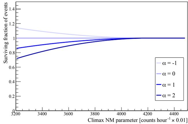
Figure 65: The function  $f_s(\alpha)$  showing an example of the parameterization of the solar activity effect by a single parameter  $\alpha$ , in the case where the sample  $s$  is the  $e$ -like up-going sample.
