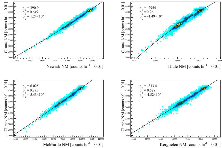
Figure 62: Fitted conversion functions between the pressure-corrected data from several NMs to the Climax neutron monitor. Each data point represents the neutron count recorded at each monitor during a given hour.
