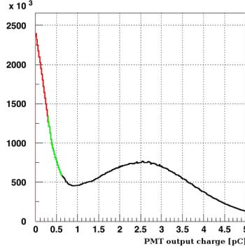
Figure 16: The single photoelectron distribution at SK, using “nickel source” data. The green part of the curve was measured by specially lowering the charge threshold of the ATM modules (see Sec. 3.3), and the red part of the curve is a simple extrapolation. [79]
