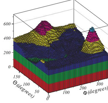
Figure 24: An example Hough-space for a ring search in SK, showing the value of a Hough parameter depending on the zenith  $\Theta$  and azimuth  $\phi$  angles from the fitted vertex, where two rings are clearly found (in this figure, the  $n_{\text{pe}}$  of the primary ring is not subtracted). [66]
