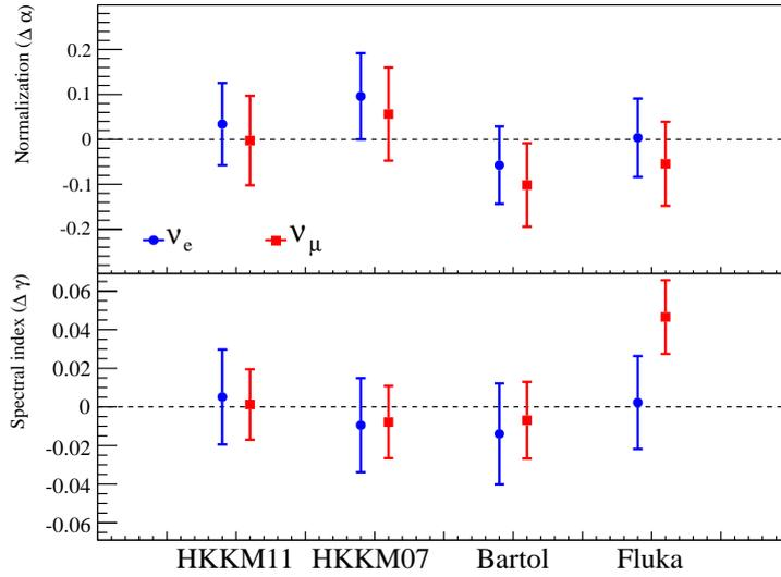
Figure 44: The best-fit and  $1\sigma$  error of the normalization and spectra index parameters  $\Delta\alpha$  and  $\Delta\gamma$ , obtained by  $\chi^2$  calculation against each model with the parameters artificially shifted.
