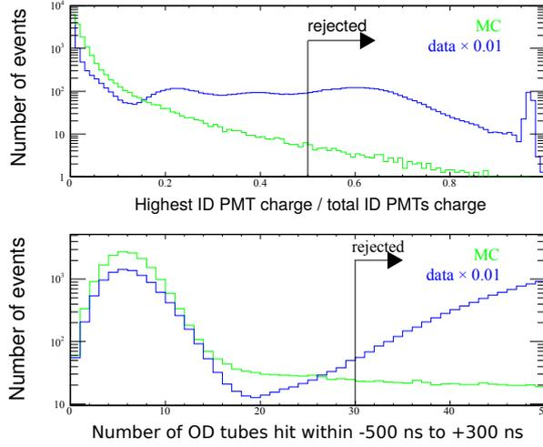
Figure 19: Distributions of the atmospheric MC and data before the FC2 cuts 3 (top) and 4a (bottom), where MC events are true high-energy FC neutrino events in the FV, and data represents the raw detector output before each cut. Note the logarithmic  $y$ -axis and the scaling factor of the data distribution. [89]
