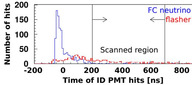
Figure 20: Comparison of a nominal FC neutrino event and a nominal flasher event, both found in SK-I data. The scanned region shows the timing region tested by the FC<sub>3</sub> cut 10. [90]
