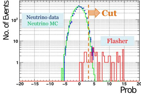
Figure 21: Comparison of the likelihood parameter “Prob” for neutrino data, MC, and hand-selected flasher events, showing the cut value. [76]
