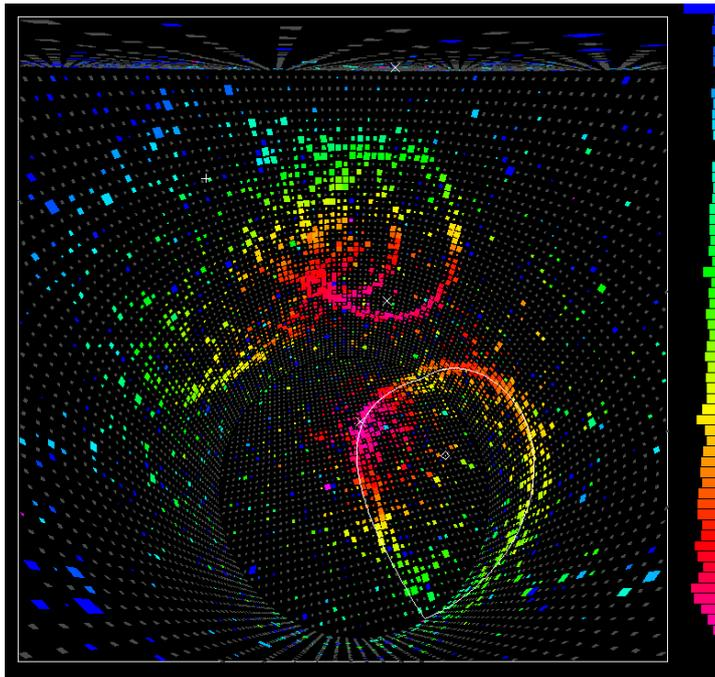
Figure 15: A three dimensional projection of a multi-ring data event. The color scale represents time over an 80 ns period, and charge is represented by the size of the square placed at each PMT position. [66]
