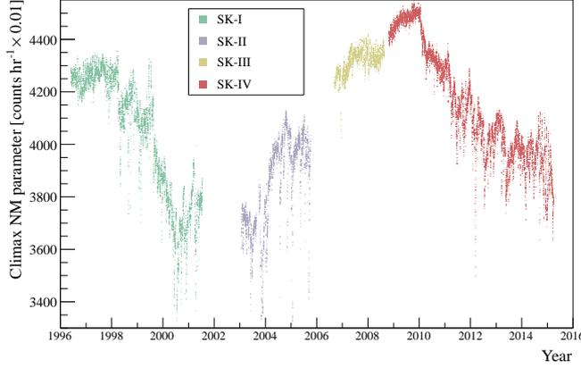
Figure 63: The values of the “Climax NM parameter” plotted over the operational history of the SK detector, where each point represents a neutrino event. Two solar maxima can be clearly seen, as can some areas where SK was not operational (such as the maintenance works between SK periods). Some sharp downward peaks can be seen, which will be analysed separately as described in Sec. 7.2.7.
