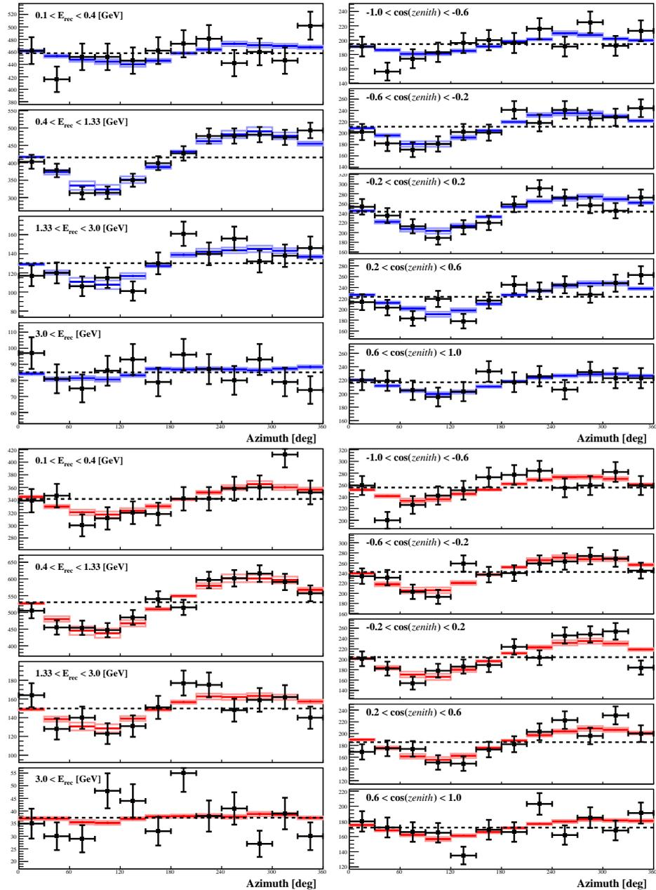
Figure 56: Single-ring e-like (top) and  $\mu$ -like (bottom) events for the SK-I to SK-IV data (error-bars) and MC (error-boxes), by reconstructed azimuthal angle. The left plots show reconstructed energy ranges summing over all zenith angles  $\theta$ , and right plots show zenith angle ranges summing over all energies  $E_{\text{rec}}$ . The plots are zero-suppressed to show the data/MC shape comparison clearly.
