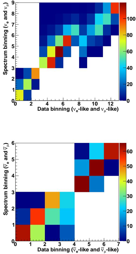
Figure 47: The initial estimation of the detector response matrix  $A_{ji}^{-1}$  for the  $\nu/\bar{\nu}$  separated unfolding, showing  $\nu$  (top) and  $\bar{\nu}$  (bottom) for SK-I.
