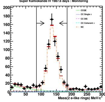
Figure 30: The  $\pi_0$  mass peak after reconstruction, from the  $\pi_0$ -like (two fitted electron ring) sample. Both the MC with interaction type breakdown, and data points with statistical error are shown.
