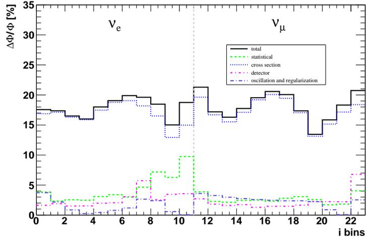
Figure 41: Breakdown of the estimated uncertainties in the measured flux values depending on each error group (statistical, detector response, neutrino cross section, neutrino oscillation, and regularization). The  $x$ -axis represents the output spectrum bins as defined in Tab. 13. The “total” histogram represents the error when all error sources are considered simultaneously.
