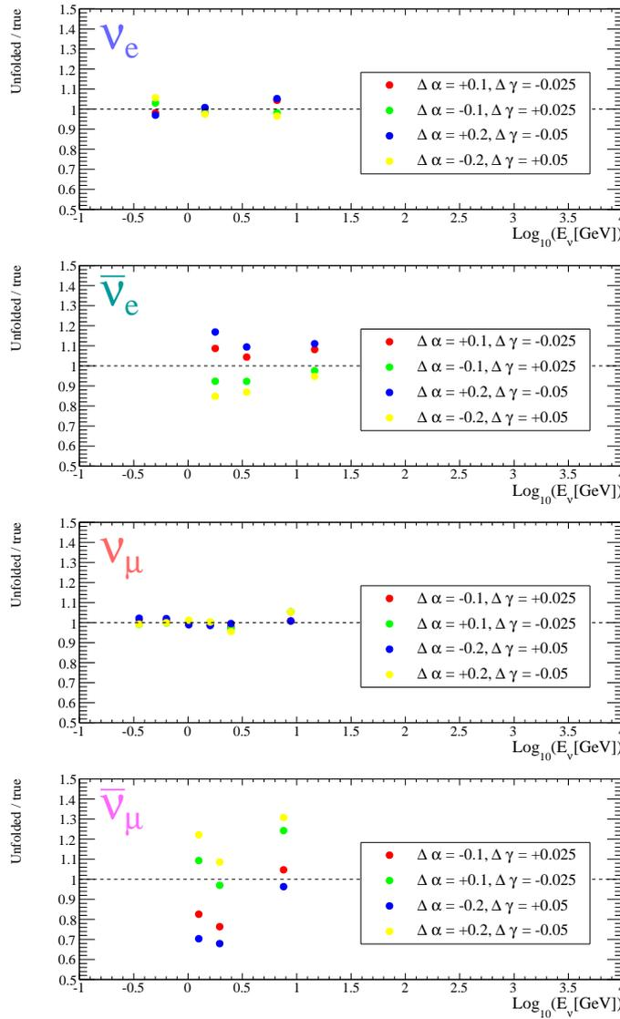
Figure 48: The regularization error estimated on the four  $\nu/\bar{\nu}$  separated samples.
