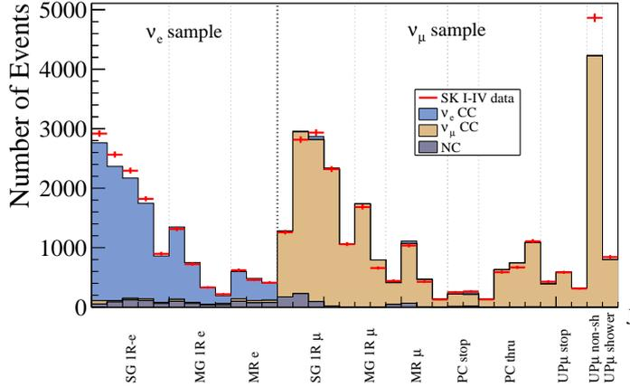
Figure 37: Number of events for each reconstructed energy bin  $M_j$  for each sample, for the entire SK-I to SK-IV period. The filled histograms are the MC truth predictions, and red represents the data counts with statistical error. Some inconsistency between the MC and data is seen, which can be accounted for within the estimated systematic errors (not plotted here).
