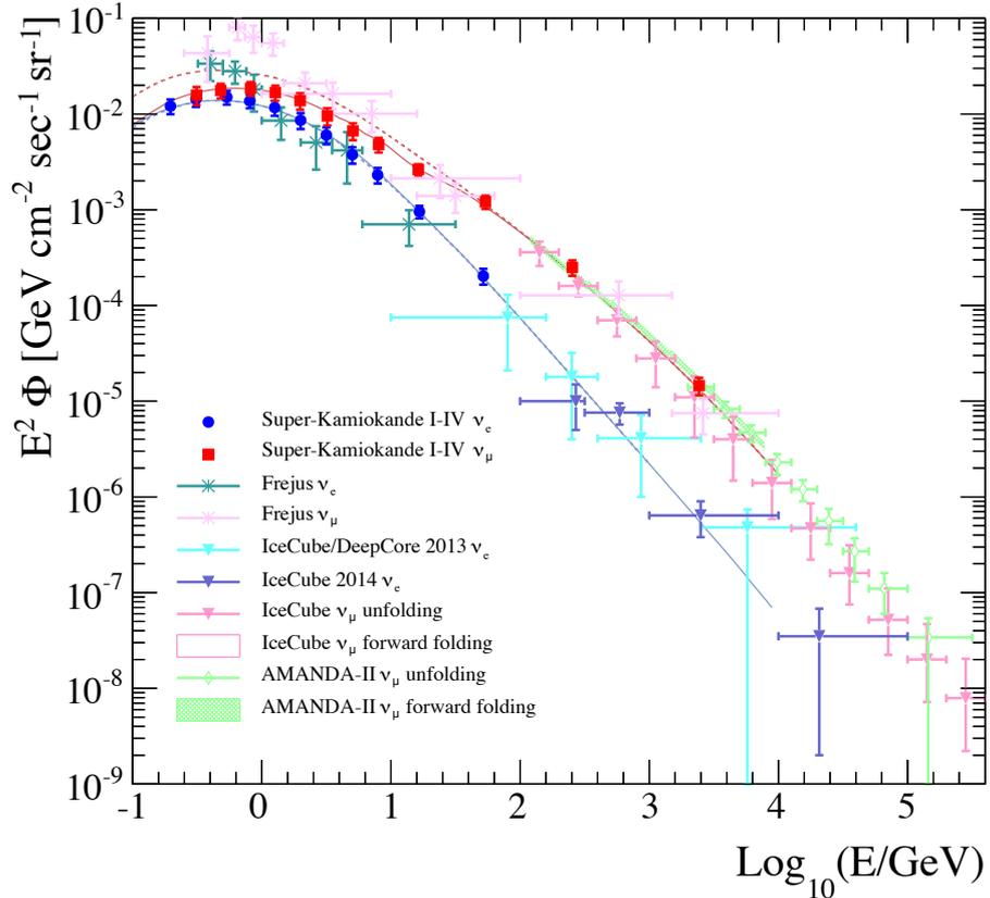
Figure 46: The measured energy spectra of atmospheric  $\nu_e$  and  $\nu_\mu$  at SK, shown in comparison to measurements by Frejus [28], AMANDA-II [29, 30], and IceCube [31, 33, 32]. The HKKM<sub>11</sub> flux curves are also shown in solid (with oscillation) and dashed (without oscillation) lines.
