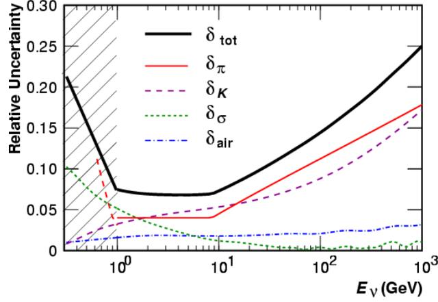
Figure 9: The estimated systematic errors on the HKKM07 model. The error sources are as follows: atmospheric density profile uncertainties  $\delta_{\text{air}}$ , mean free path (cross-section) uncertainties  $\delta_{\sigma}$ , kaon flux uncertainties  $\delta_K$ , pion flux uncertainties  $\delta_{\pi}$ , and total uncertainty  $\delta_{\text{tot}}$ . [75]
