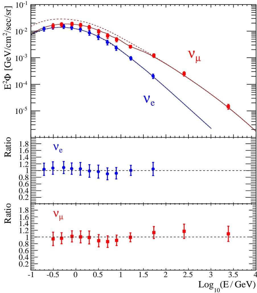
Figure 42: The measured flux energy spectra, using all SK-I to SK-IV data, for  $\nu_e$  (blue) and  $\nu_\mu$  (red). The flux values are shown multiplied by  $E^2$ , following a common convention. Error bars include all statistical and systematic uncertainties. The curves show the HKKM11 [19] model's prediction with (solid) and without (dashed) neutrino oscillation (same color scheme). The lower part of the figure shows the ratio of data / HKKM11 prediction.
