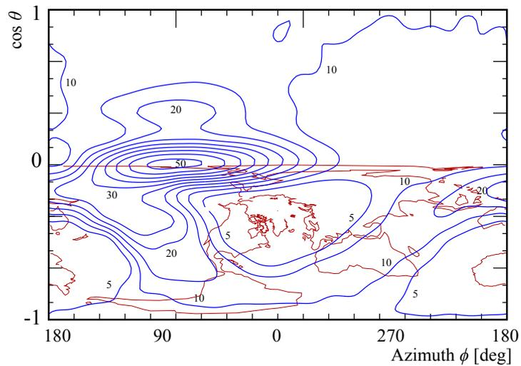
Figure 7: Contour map of the rigidity cutoff, seen from the perspective of the SK detector. The labeling of the azimuth angle  $\phi$  and zenith angle  $\theta$  is the same as in Sec. 6.2. The units represent the rigidity cutoff in GV (e.g. for a proton with a charge of  $+e$ , this is the required energy in GeV to pass the cutoff). [67]
