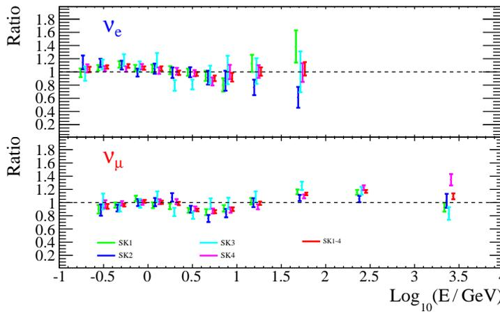
Figure 45: Flux ratio to the HKKM11 model for each SK period. Error bars include only statistical uncertainty in this figure.
