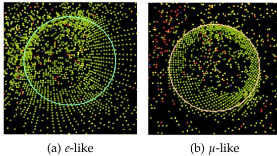
Figure 26: An example comparison between an  $e$ -like and a  $\mu$ -like ring pattern of roughly the same energy, where each dot represents a hit PMT, colored corresponding to the detection time. [66]
