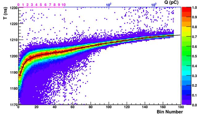
Figure 17: Example time vs. charge distribution map (TQ map) for an SK ID PMT. The upper x-axis showing the actual charge is a combination of linear and log scales, the black line represents a series of fitted polynomial functions, and the color scale is arbitrarily normalized. [79]
