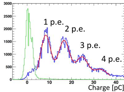
Figure 13: Example raw charge outputs from a modern PMT, showing “dark rate” data (green), charge outputs during exposure to a light source (blue), and fitted  $n_{pe}$  distributions (red). The dark rate refers to random outputs in the absence of a light source, coming from e.g. thermionic emission. Shown for illustrative purposes only (not used in Super-Kamiokande). [76]
