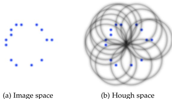
Figure 23: Illustration of the principle of the circular Hough transform, where blue represents image intensity, and black represents the Hough parameter intensity. The recorded image is shown in (a), and the transformation to circular Hough space in (b), where the location of the darkest point is the estimated centre of the fixed width circle (the image itself is overlaid in the Hough space, for illustrative purposes).
