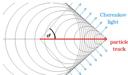
Figure 10: Cherenkov light production by a charged particle track. Dotted angles represent right angles. [55]
