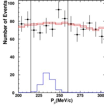
Figure 2: An example of the atmospheric neutrino flux as a background source – data from the search for proton decay via the mode  $p \rightarrow \nu + K^+$  at Super-Kamiokande. The reconstructed muon momentum distribution is shown. The red boxes correspond to the atmospheric neutrino simulation, and the blue line histogram is the expected proton decay signal.
