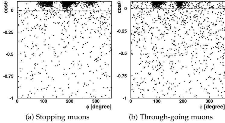
Figure 34: Fitted stopping and through-going muon data for SK-I, where  $\phi$  is the azimuthal angle and  $\theta$  is the zenith angle. Mostly up-going ( $\cos \theta < 0$ ) neutrino-induced events are shown, although in the  $0 < \cos \theta < 0.1$  range some clusters of the cosmic-ray background are clearly visible.
