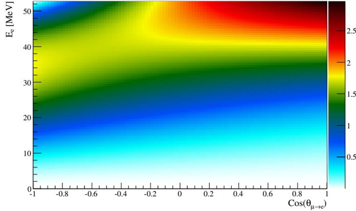
Figure 52: The predicted decay rates for the Michel decay  $\mu^- \rightarrow e^- + \bar{\nu}_e + \nu_\mu$  ( $\mu^+ \rightarrow e^+ + \bar{\nu}_\mu + \nu_e$ ). Here  $E_e$  is the electron (positron) energy, and  $\theta_{\mu \rightarrow e}$  is the inner angle between the muon *spin* and electron (positron) *momentum*. Column normalized.
