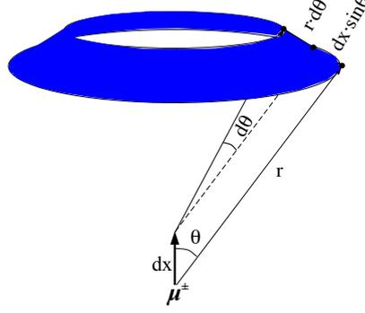
Figure 27: Diagram showing the calculation of Cherenkov light emission from a muon track (variables are explained in the text). [66]
