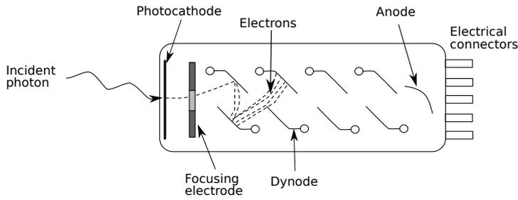
Figure 11: Basic operating principle of the photomultiplier tube. [55]
