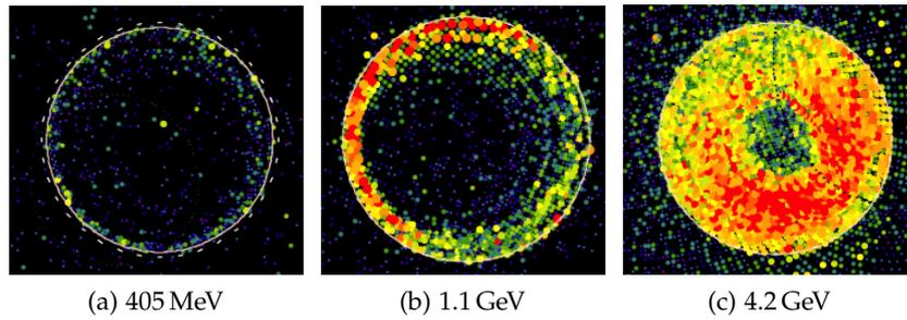
Figure 29: An example comparison between ring patterns for a muon of varying energy, where the size and color of the dots represent the hit charge of each PMT. [66]
