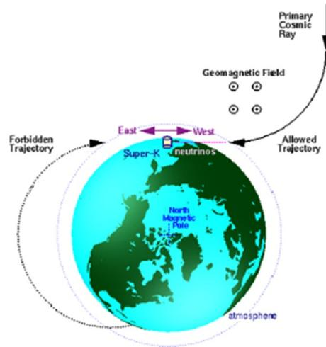
Figure 6: Illustration of the rigidity cutoff effect, for two primary cosmic ray collisions that could result in neutrino events at Super-Kamiokande. After tracing backwards in time, only one cosmic ray passes the rigidity cutoff test. [66]
