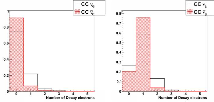
Figure 33: The true neutrino purities of the multi-GeV single-ring  $e$ -like (left) and  $\mu$ -like (right) samples, as a function of the number of tagged Michel electrons (or positrons). The histograms are normalized to unity, and the wrong-flavour background of each sample is not plotted. [84]
