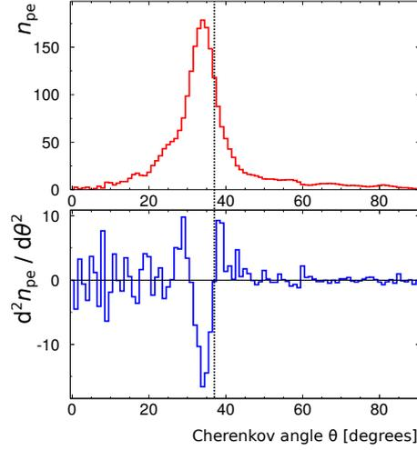
Figure 22: An example distribution of observed charge depending on the Cherenkov angle  $\theta$ , and its second derivative, for a given ring position and direction. The dotted line indicates the fitted edge of the ring. [66]
