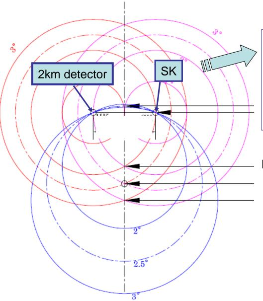
The beam may not be identical between SK and 2KM (Anselmo's talk). → Left-right monitor at the 280m hall. (Left-right monitor at the 2km site is impossible.)
