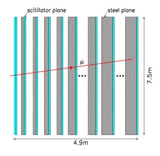
The MRD consists of 22 steel plane followed by a scintillator plane. Before it are placed two scintillator planes. The size of the MRD is  $7.5 \text{ m} \times 7.5 \text{ m} \times 4.9 \text{m}$ . The first two steel plates are of 2.5cm thick, the next two planes have thickness of 5cm, the next ten layers are of 10cm thick and the last eight are of 20cm.
