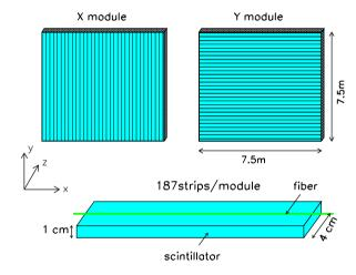
Each scintillator plane is made up to 187 strips, each 4 cm wide by 1cm thick and 750cm long. The orientation of the strips alternates  $\pm 90^{\circ}$  in successive planes (X and Y modules).
