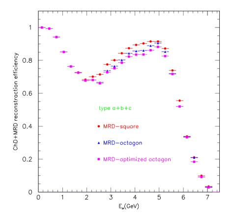
Efficiency of (MRD I) configuration is diminished of 4% and (MRD II) - of 6%.
