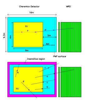
To study the perfomance of the MRD charge-current neutrino events were simulated in fiducial volume of 1kt detector. It was assumed that K2K MRD square steel sheets can be used for 2km MRD.
