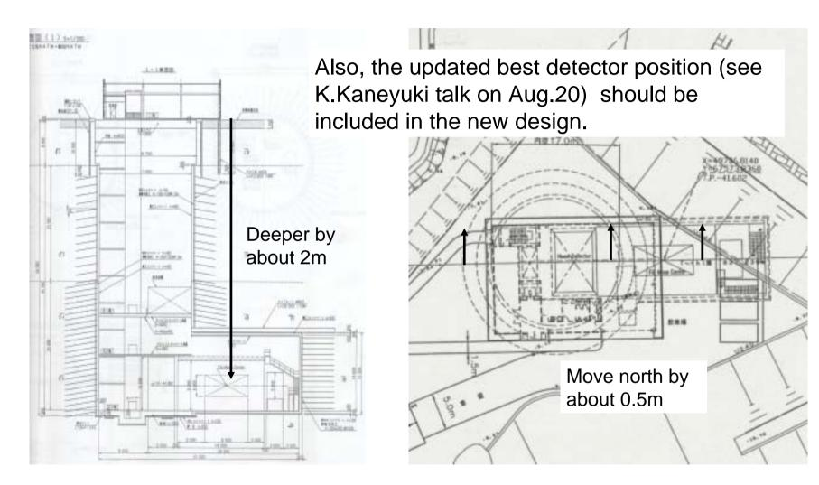
• We have contacted the facility designing company again. They will re-design the experimental hall with smaller vertical tunnel.
