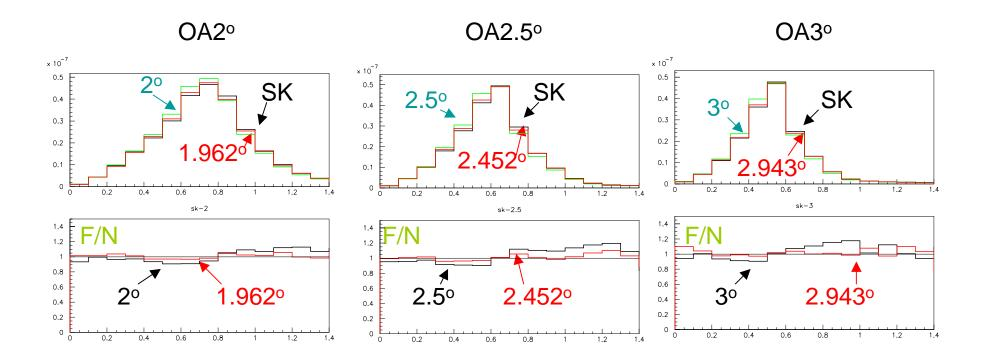
Far/Near ratio is improved by taking into account the v beam production point.
