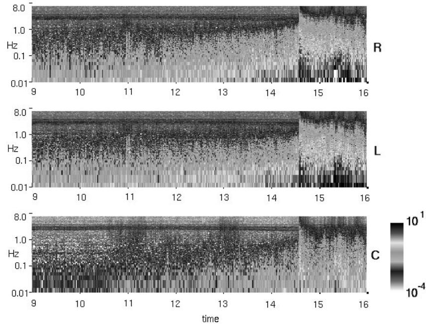
**Fig. 3.** Time profile of power spectra. The shock arrival time was 1435 UT. The three panels respectively show dynamic spectra of right, left and compressional component. Horizontal lines above 1 Hz are due to artificial noise and not natural.
