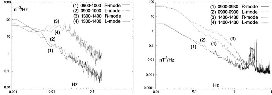
**Fig. 2.** (a) The power spectra of the lower frequency range. (b) The power spectra of the higher frequency range. Peaks above 1 Hz are artificial noise and not natural. In (a), spectra are calculated by using 256 point FFT of 3-second-averaged FX data (the degrees of freedom is 4); In (b), spectra are calculated by using 2048 point FFT of original 16 Hz FX data (the degree of freedom is 11).
