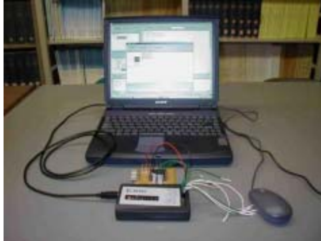
Fig. 1. Download process from a PC to the chip via a MultiLINX.
