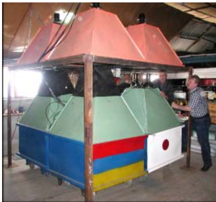
Fig. 1. The Solar neutron Telescope SNT1 at Mt. Aragats (3250m). The detector consists of two layers of plastic scintillators for anti-coincidence (to reject charged particles) and thick (60cm) plastic scintillator to convert neutrons into protons and measure the energy of those protons. At present the SNT1 can measure the direction of protons in 9 directions.
