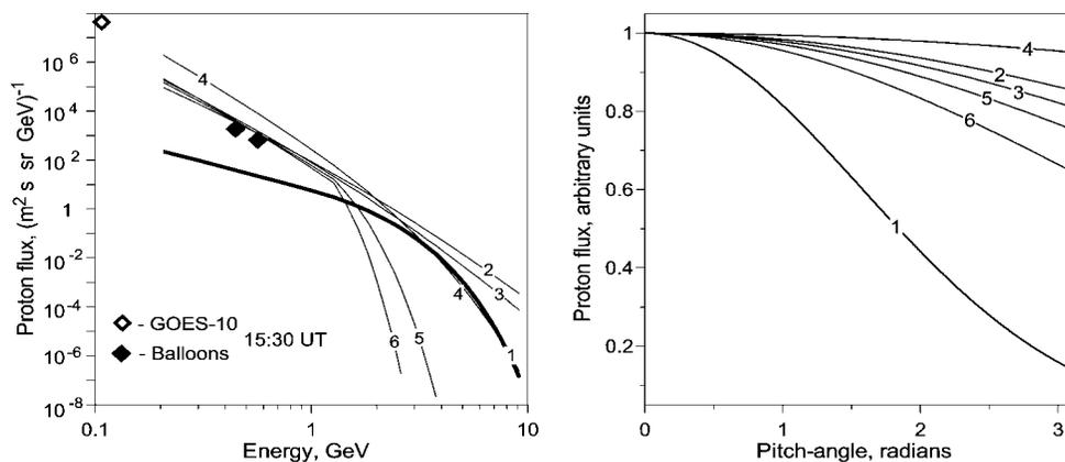
**Fig. 1.** a: derived energy spectra of RSP, b: pitch-angle distributions (PAD) at different moments of time on 14 July, 2000 that are: 1-10.40, 2-11.05, 3-11.30, 4-12.00, 5-12.30, 6-13.00. Thick line in Fig.1a is spectrum of prompt component of RSP. The balloons and GOES 10 points are data of direct solar proton measurements.
