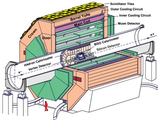
**Fig. 1.** The L3 spectrometer. Only the muon detectors, the magnet and the scintillator tiles were used in this experiment.
