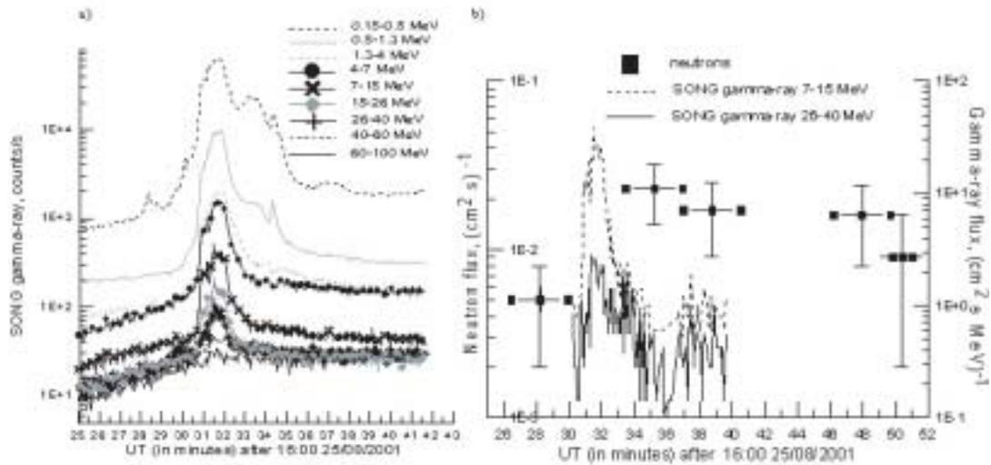
**Fig. 1.** The count rate of gamma rays by SONG (a) and solar neutron and gamma-ray flux (b) on CORONAS-F during the solar flare on August 25, 2001.
