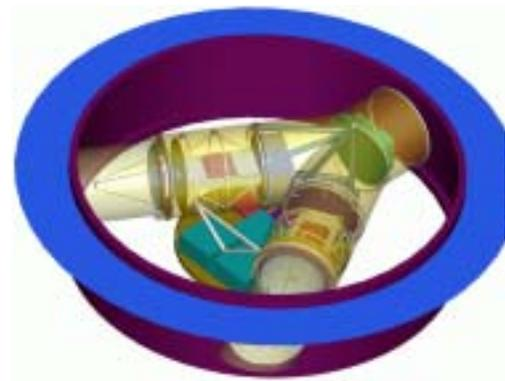
**Fig. 2.** View of LISA spacecraft, housing two optical assemblies. The solar panel at top not shown.
