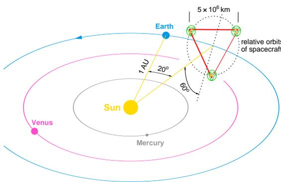
**Fig. 1.** Orbits of the three spacecraft of LISA, trailing the Earth by  $20^\circ$ . The triangle arms are scaled by factor 10.
