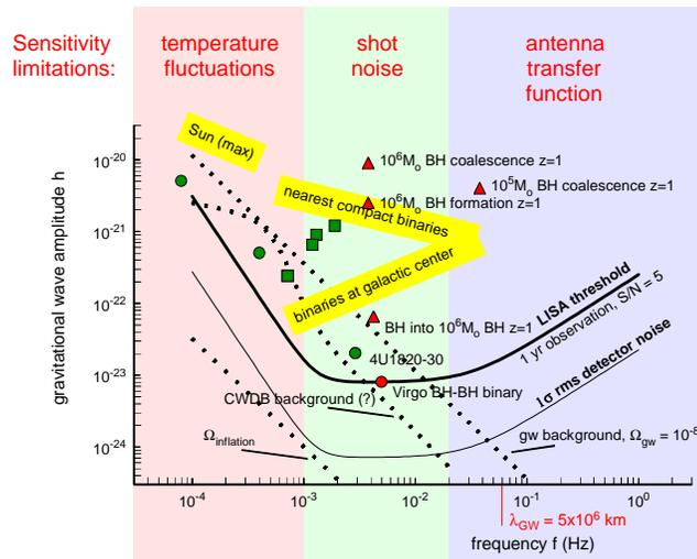
**Fig. 3.** Sensitivity of LISA: the heavy curve “LISA threshold” represents the signal strength that would provide a signal-to-noise ratio of 5 when averaged over one year.
