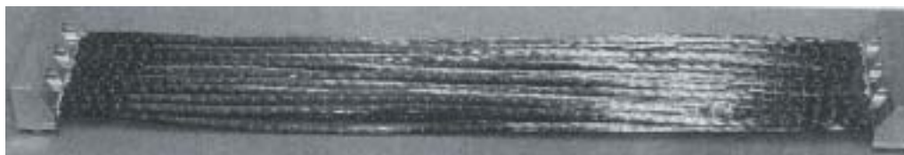
Fig. 2. K1100 graphite fiber thermal strap assembly [6]
