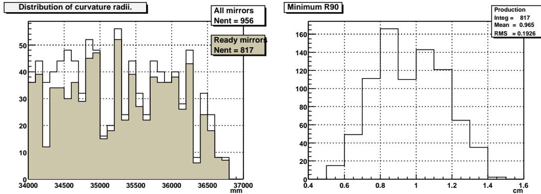
**Fig. 2.** Distribution of the curvature radii for all the 956 mirrors (*left*). Distribution of  $R_{90}$  for the measured production mirrors (*right*).
