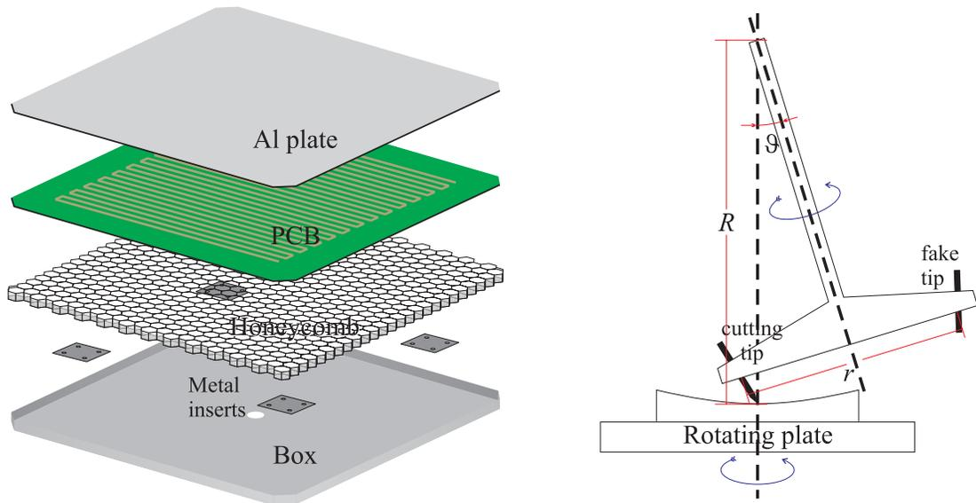
**Fig. 1.** Exploded view of the *raw-blank* structure (*left*). Sketch of the milling tool and the rotating table (*right*).
