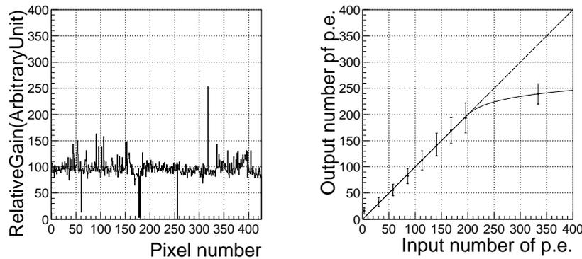
**Fig. 1.** Left: Hardware gain distribution. We can estimate the absolute number of incident photoelectrons (p.e.) by assuming a Poisson distribution. Right: output p.e. versus input p.e. The linearity is maintained up to about 200 p.e. and the dynamic range after software corrections is about 250 p.e.
