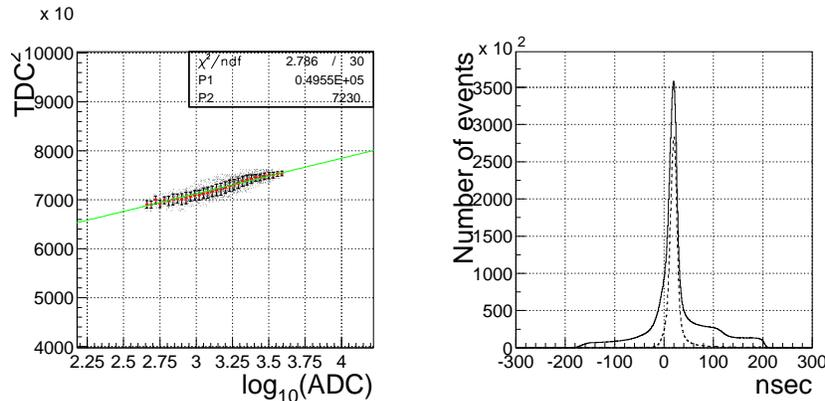
**Fig. 2.** Left:  $(TDC)^2$  versus  $\log(ADC)$ . This distribution was fitted with a line. Right: timing distributions of a pixel in a typical observation. After the time-walk correction, the solid line is for all triggered pixels and the dotted line is after a further off-line selection (dotted line).
