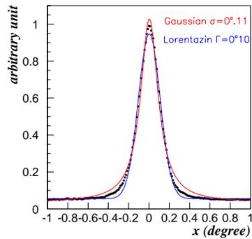
**Fig. 5.** Spot-size of the second telescope.
