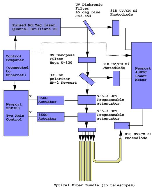
**Fig. 2.** Schematic Central Optical Injection for VERITAS
