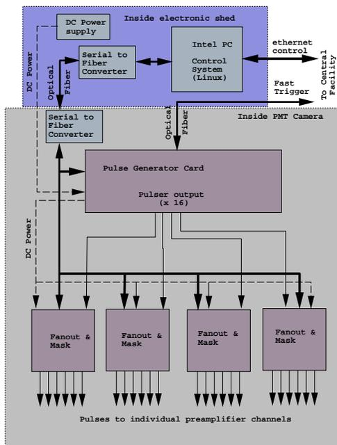
**Fig. 1.** Schematic Electronic Charge Injection scheme for VERITAS
