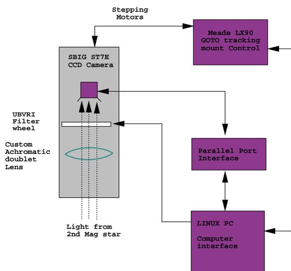
**Fig. 3.** Schematic drawing of Star Tracking Atmospheric Monitoring system for the VERITAS observatory.
