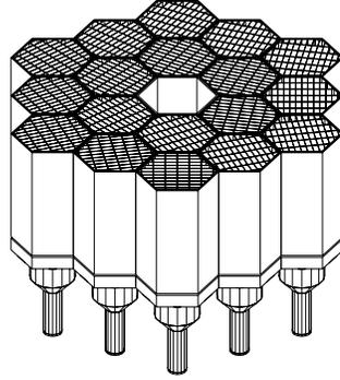
**Fig. 1.** Schematic diagram of the main HXMT detector.
