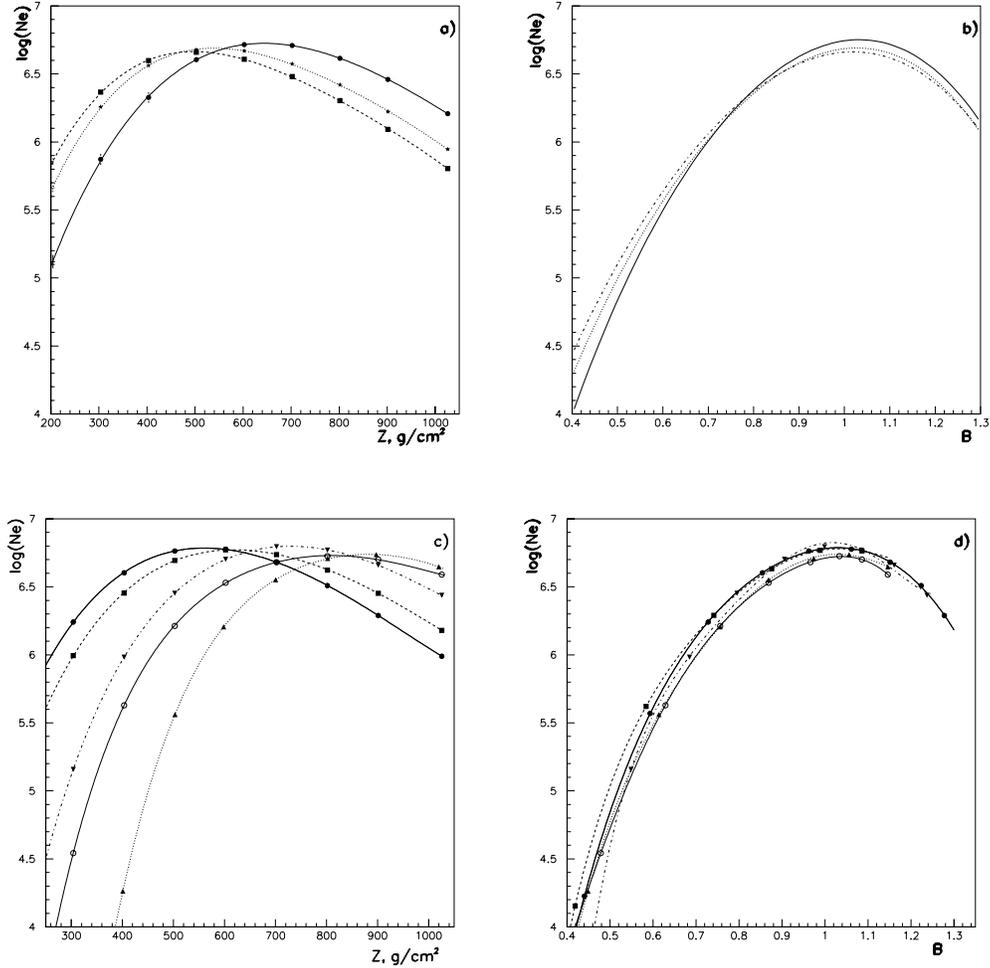
**Fig. 1.** a) mean cascade curves of EAS induced primary cosmic proton (solid), oxygen (dotted) and iron (broken) at primary energy of  $10^{16} eV$ ; b) mean  $BL$ -curves for the same EAS; c) cascade curves of five individual showers induced  $10^{16} eV$  primary cosmic proton; d)  $BL$ -curves for the same five showers.
