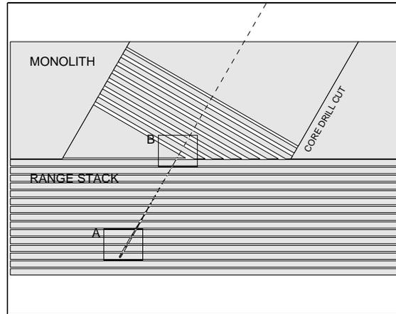
**Fig. 1.** RIO block diagram showing the monolith above and range stack below. The trajectory of a sample cosmic ray is shown as a dashed line.
