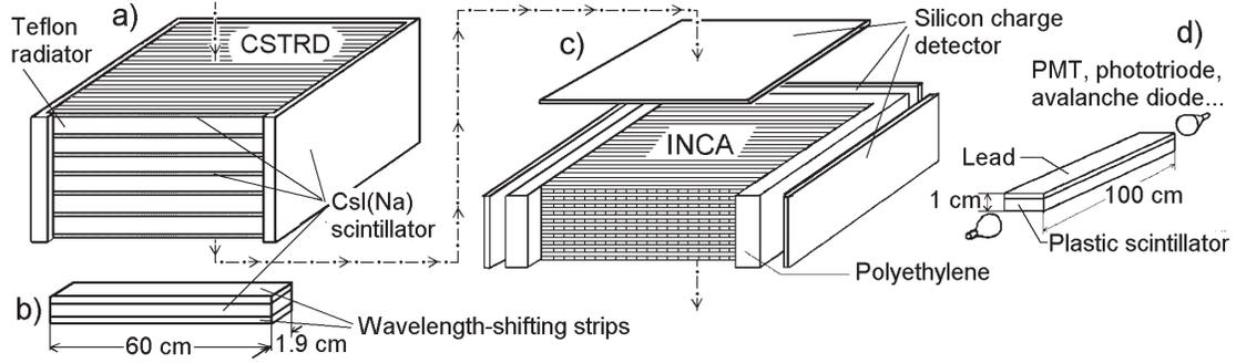
**Fig. 1.** Schematic of the INTREPID instrument. Certain of the elements are not shown for simplicity.
