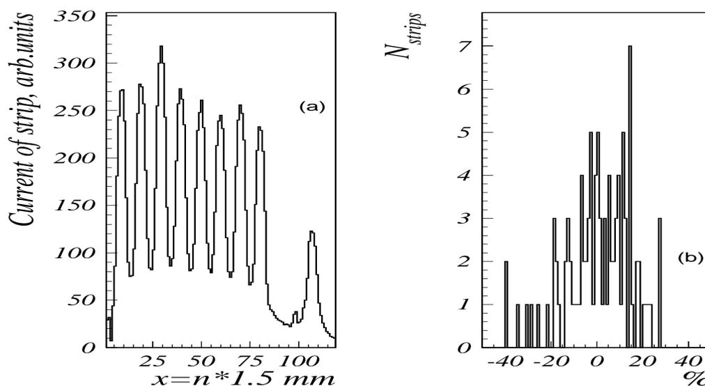
**Fig. 2.** Left - signals of test with  $\beta$ -source  $^{90}\text{Sr}$  moving across a strip plane. Right - dispersion of the average relative amplitudes of 192 strips.
