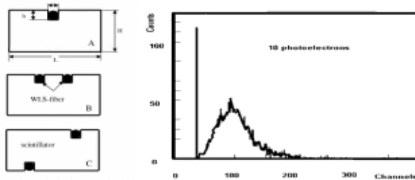
**Fig. 1.** Left - transverse section of scintillator strips with WLS fibers:  $H=5 \text{ mm}$ ,  $L=7.5 \text{ mm}$ , fiber diameter  $d=1 \text{ mm}$ . Right - typical spectrum of cosmic muons .
