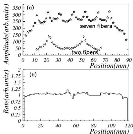
**Fig. 3.** a) Thin scintillator test with  $\beta$ -source  $^{90}\text{Sr}$ . b) The relative light output of strips measured before and after mechanical tests.
