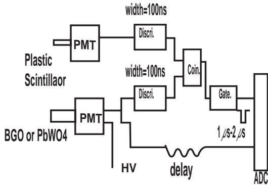
**Fig. 3.** An experimental setup for the muon measurement. All scintillators were wrapped by the Teflon sheet with reflectivity  $\geq 90\%$
