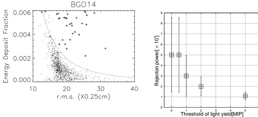
**Fig. 1.** The energy deposit fraction in the 14th BGO-layer as a function of the spread of the shower. Plus sign shows 10 TeV protons and dot sign shows 4 TeV electrons.
