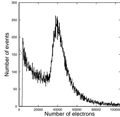
**Fig. 6.** The light yield of BGO by cosmic muon measured with PD. Solid curve shows a fitting function by sum of a landau and an exponential distribution.
