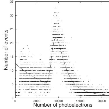
**Fig. 4.** The light yield of BGO by cosmic muon measured with PMT as shown in Fig. 3. Solid curve shows a fitting function by sum of a Landau and a exponential distribution.
