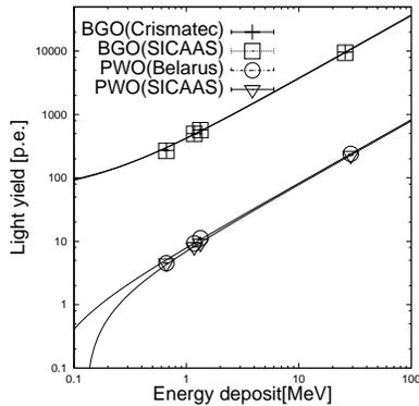
**Fig. 5.** The light yield of BGO and  $\text{PbWO}_4$ . The solid lines show the linear functions.
