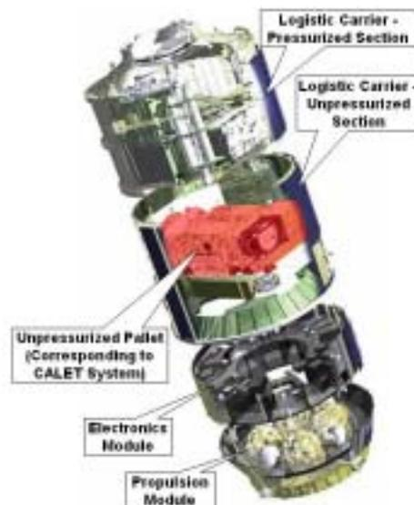
**Fig. 3.** H-II Transfer Vehicle (HTV)
