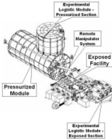
**Fig. 1.** The Japanese Experiment Module (JEM) on the International Space Station
