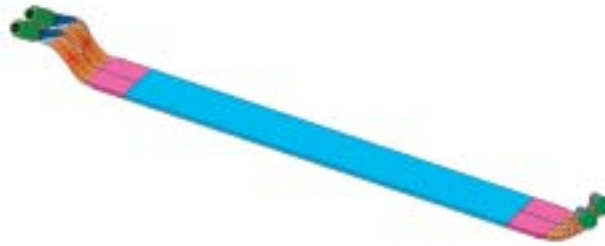
Fig. 2. A complete TOF counter with 2 + 2 PMT and curved light guides.
