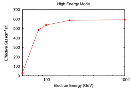
**Fig. 2.** Energy dependence of the geometrical factor for electrons in the HE-mode by simulation.
