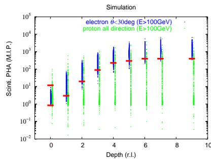
**Fig. 1.** Simulated shower development of electron and protons over 100 GeV. Lines denote discrimination levels.
