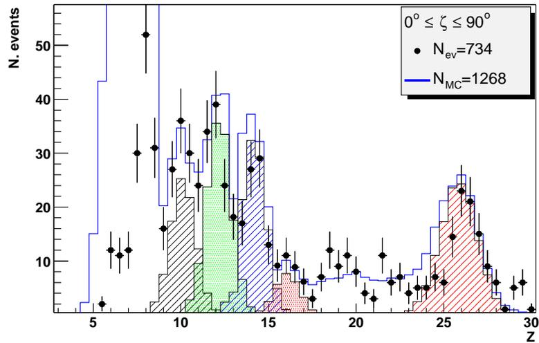
**Fig. 3.** The comparison of data (points) to MonteCarlo (blue line) for events with charge number  $5 \leq Z \leq 32$ . The dashed histograms indicate the MonteCarlo events generated with  $Z=10(\text{Ne})$ ,  $12(\text{Mg})$ ,  $14(\text{Si})$ ,  $16(\text{S})$  and  $26(\text{Fe})$
