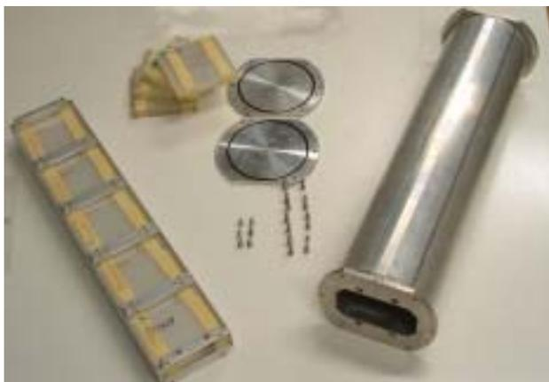
**Fig. 1.** The stacks, the tray and the pressurized cylinder that constitute the basic unit of CAKE
