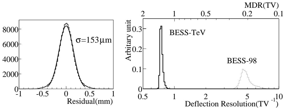
**Fig. 3.** Residual distribution of ODC **Fig. 4.** Distribution of the deflection resolution. Each area of the histogram is normalized to unity.
