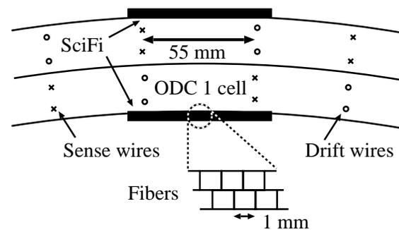
**Fig. 2.** Schematic view of SciFi mounted on ODC
