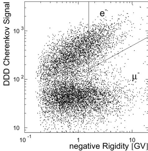
**Fig. 2.** Separation and selection of  $e^-$  with DDD Cherenkov counter.
