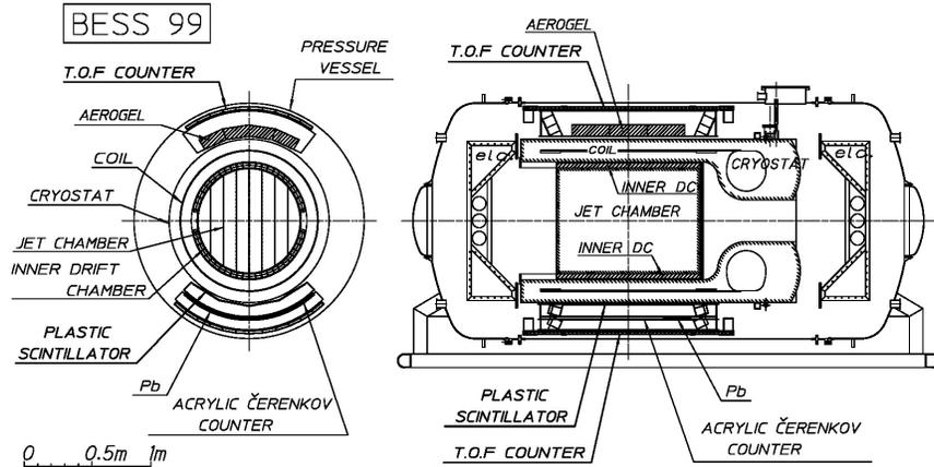
**Fig. 1.** Cross-sections of BESS-1999 Instrument.
