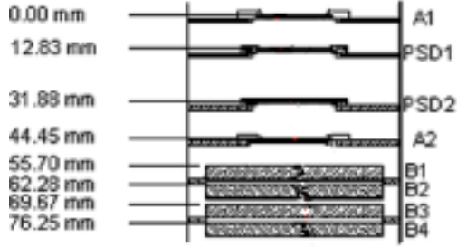
Fig. 1. MARIE detector stack showing the position of the detectors.
