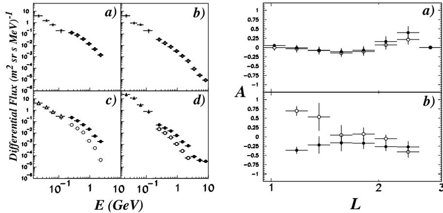
**Fig. 3.** Left: Differential flux of  $e^+$  (a, c) and  $e^-$  (b, d) for  $L < 1.2$ . Stars and triangles show the MARYA [4] data outside and inside the SAA, respectively. Full and empty circles show the AMS QT and ST fluxes inside the SAA. Crosses refer to the QT fluxes measured outside the SAA. Right: East/West asymmetry of integral  $e^-$  (empty dots) and  $e^+$  (full dots) fluxes. QT and ST components are shown in a) and b) respectively.
