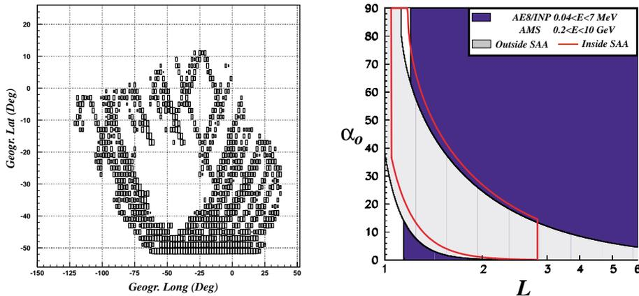
**Fig. 1.** Left: the geographical region corresponding to the SAA measurements. Right: the field of view of AMS in the  $(L, \alpha_0)$  parameter space.
