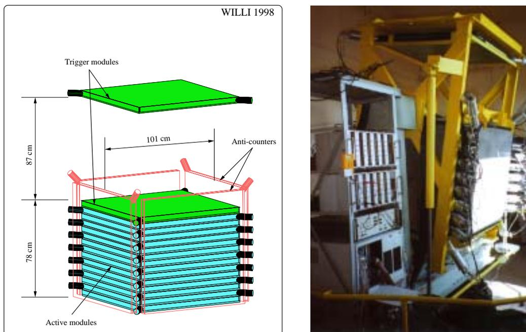
**Fig. 1.** Schematic view of the original WILLI detector (left) and the configuration in a rotatable frame (right)
