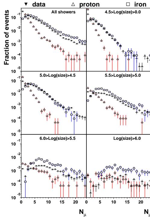
**Fig. 1.** Multiplicities observed in the muon detector, for all showers and for five selected shower ranges.
