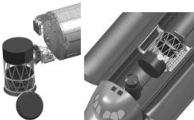
Fig. 2. EUSO on-orbit and launch configurations (courtesy of Alenia Spazio).
