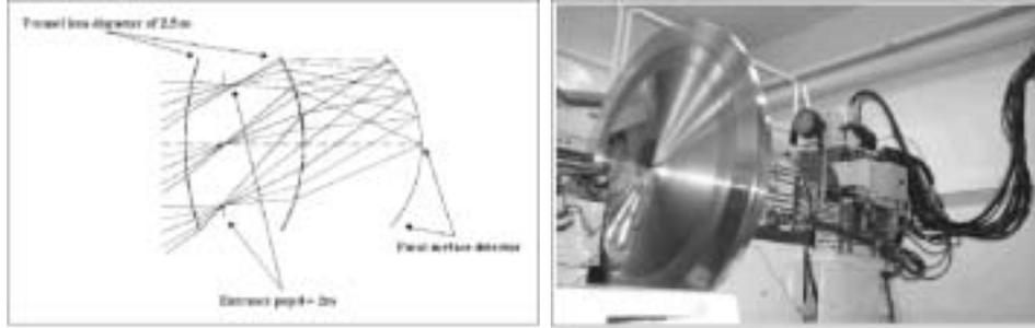
**Fig. 2.** Reduced scale prototype unit of the EUSO Fresnel lenses produced at the Optics Centre of the University of Alabama.
