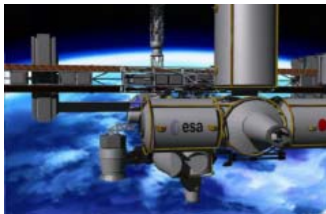
Fig. 4. EUSO is the cylindrical structure attached to the left side of ESA's Columbus External Payload Facility. The docking port for the Space Shuttle and the Japanese module can be seen to the right of the Columbus module.
