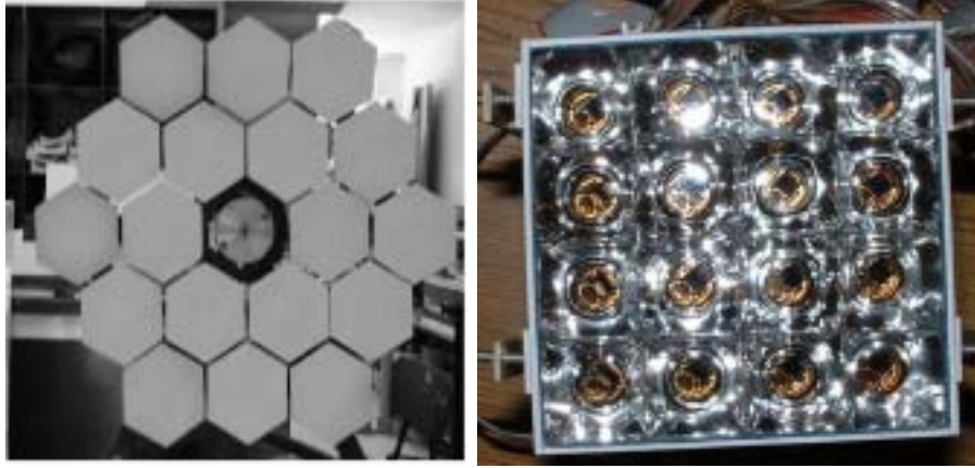
Fig. 1. Segmented telescope with 19 mirrors (left) and photosensor camera (right).
