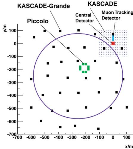
Fig. 3. Layout of the multi-detector experiment KASCADE-Grande.
