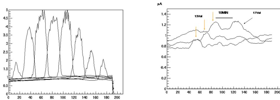
**Fig. 1.** The first stars signals seen by the FD Optical Current Monitor on June 25, 2001. The horizontal scale is the number of 20 sec interval. A star takes about 6 min to traverse a PMT along its diameter. The fluctuations at the top do not seem compatible with Poisson statistics. The vertical scale is mean anode current in  $\mu\text{A}$ .
