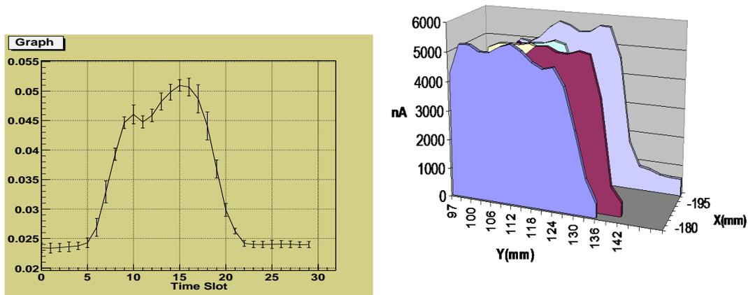
**Fig. 3.** The average shape of star signals on the same PMT of 10 different nights (left) shows the photocathode anisotropy in one of the FD PMTs. The right panel shows the photocathode response obtained at the Lab making an xy scan.
