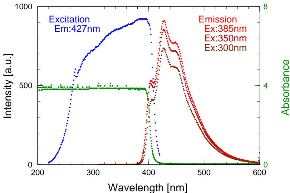
**Fig. 4.** Fluorescent/absorption spectra of the hot-pressed POPOP/polystyrene film.
