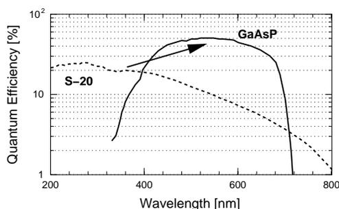
**Fig. 1.** Example of quantum efficiency for bi-alkali and GaAsP photocathodes.
