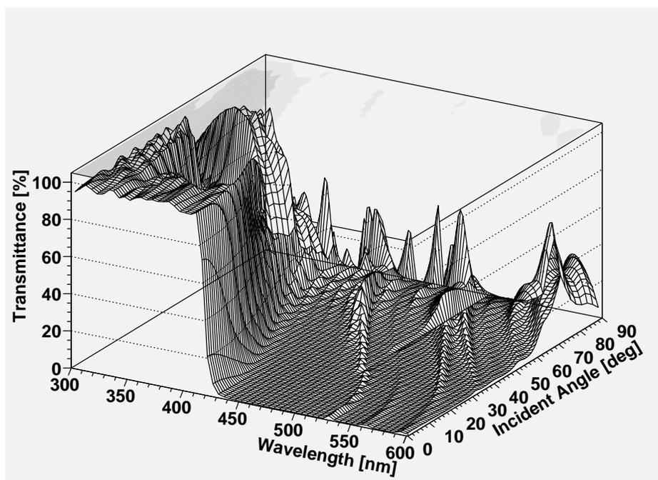
**Fig. 3.** Designed transmittance of a dichroic mirror.
