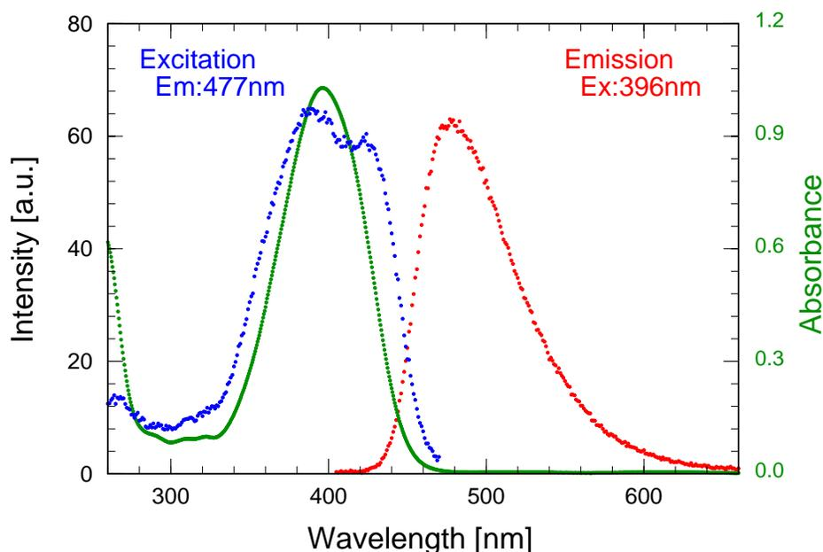
**Fig. 5.** Fluorescent/absorption spectra of the spin-coated Coumarin152A/PMMA film.
