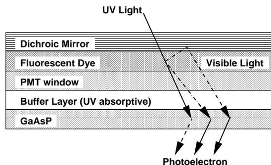
**Fig. 2.** Conceptual design to use a GaAsP photocathode in near-UV.
