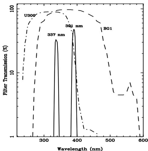
**Fig. 1.** Transmittance of the filters used in the measurements presented in the paper.
