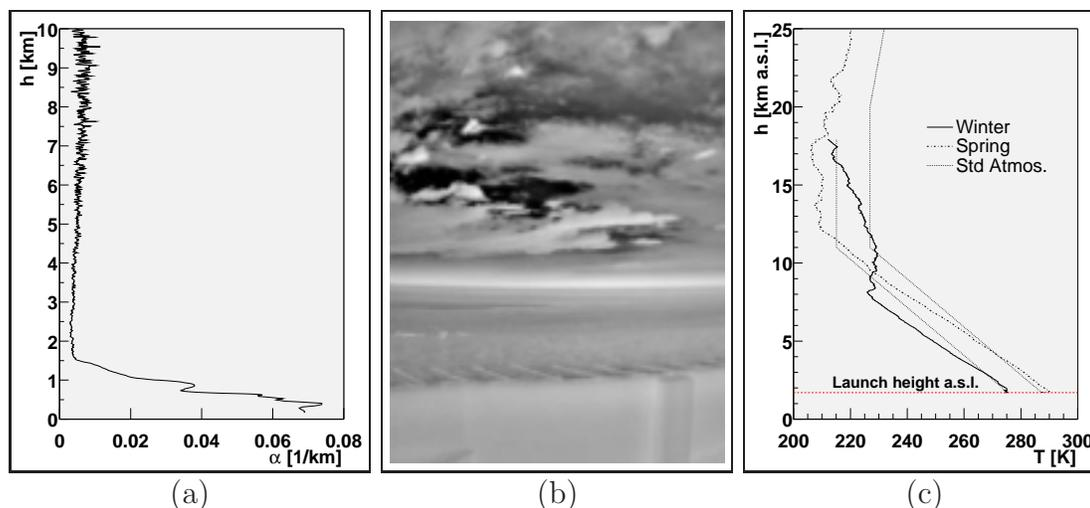
**Fig. 1.** (a) Aerosol extinction coefficient as a function of height measured with the LIDAR system at the Los Leones site. (b) Sky picture of the field of view of one of the telescopes at the Los Leones site. (c) Temperature profiles measured with radiosondes in two different seasons over the Coihueco site.
